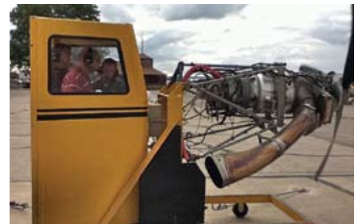
Spokane Turbine Center students practice engine starts, adjustments and tests on a working Pratt and Whitney turbine engine.
